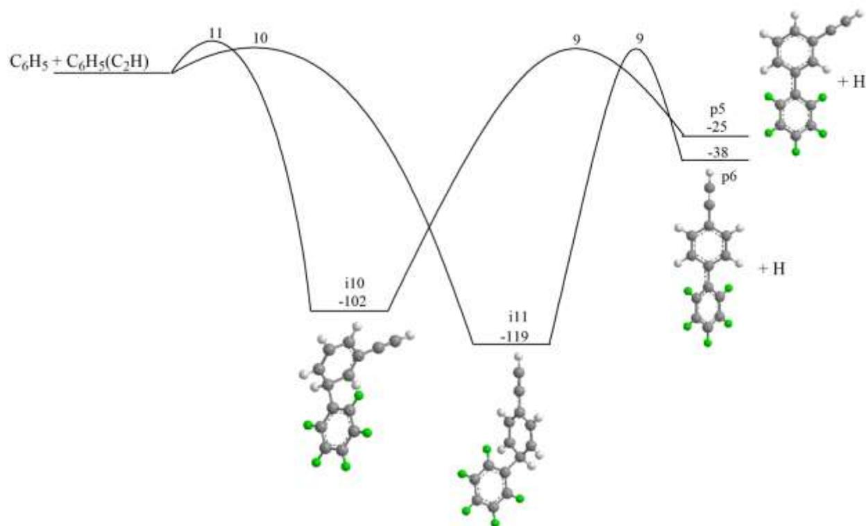
Figure 7: Schematic representation of the  $C_6D_5C_8H_6$  potential energy surface (PES) accessed via the reaction of D5-phenyl ( $X^2A_1$ ) with phenylacetylene ( $X^1A_1$ ). (A) Phenyl addition to the acetylic group of phenylacetylene, (B) Phenyl addition to the ortho carbon of phenylacetylene molecule, (C) Phenyl addition to the meta and para carbons of phenylacetylene. Atom designations: carbon – grey, hydrogen – white, deuterium – green, energy is in  $\text{kJ mol}^{-1}$ .
