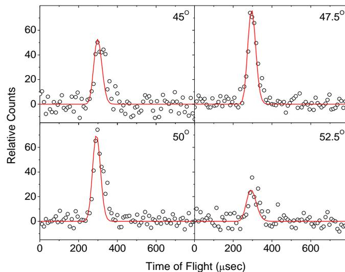
Figure 1: Time-of-flight data at  $m/z = 183$  ( $C_{14}D_5H_5^+$ ) recorded for the reaction of D5-phenyl with phenylacetylene at various laboratory angles at a collision energy of  $120.7 \text{ kJ mol}^{-1}$ . The circles represent the experimental data, and the solid line represents the fit.
