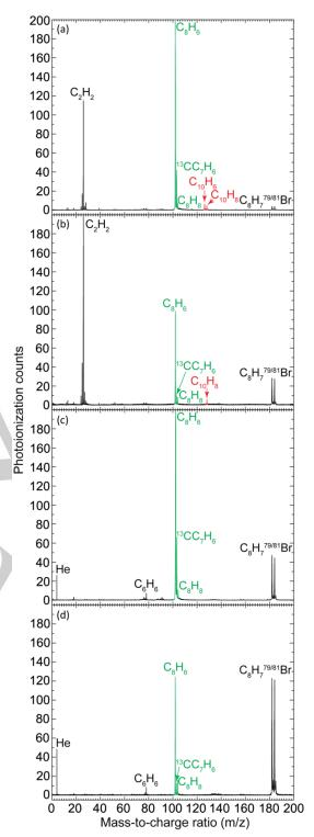
Figure 1. Mass spectra recorded at a photoionization energy of 9.50 eV for species formed via the styrenyl in acetylene (a) and *ortho*-vinylphenyl in acetylene systems (b). Spectra for acetylene replaced with helium are shown in (c) and (d), respectively. Key product isomers are labelled in red and green. Ions from acetylene and helium originate from higher harmonics.
