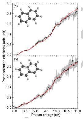
Figure 2. Photoionization efficiency (PIE) curves recorded at *m/z* 128 in the styrenyl with acetylene (a) and *ortho*-vinylphenyl with acetylene (b) systems. The black line shows the experimental curve with the uncertainty defined as the gray area. The red lines indicates the referencene PIE curve for naphthalene.
